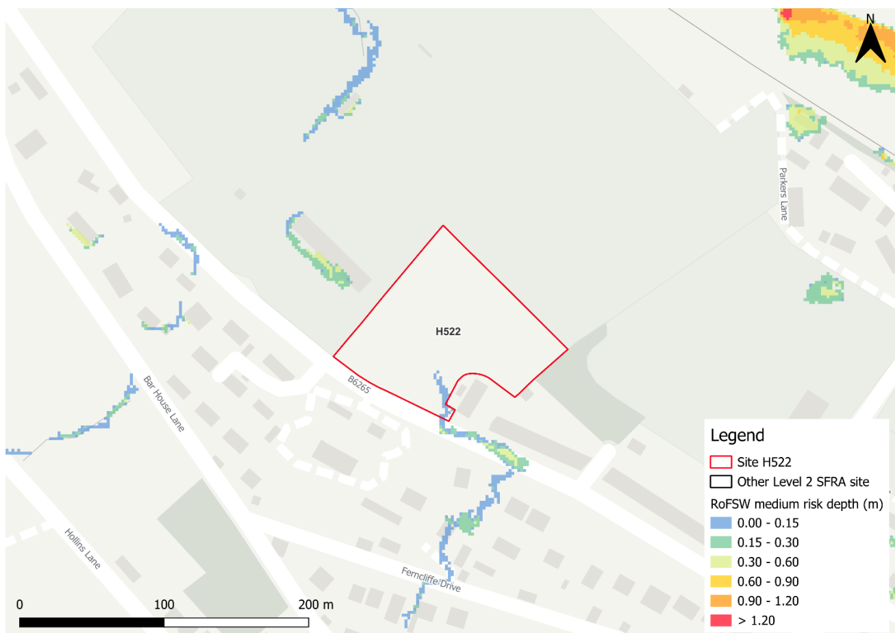
Figure 2-18: Medium risk event surface water flood depths within H522 (Risk of Flooding from Surface Water)
