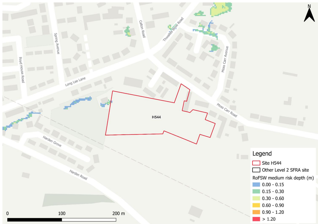
Figure 2-22: Medium risk event surface water flood depths within H544 (Risk of Flooding from Surface Water)
