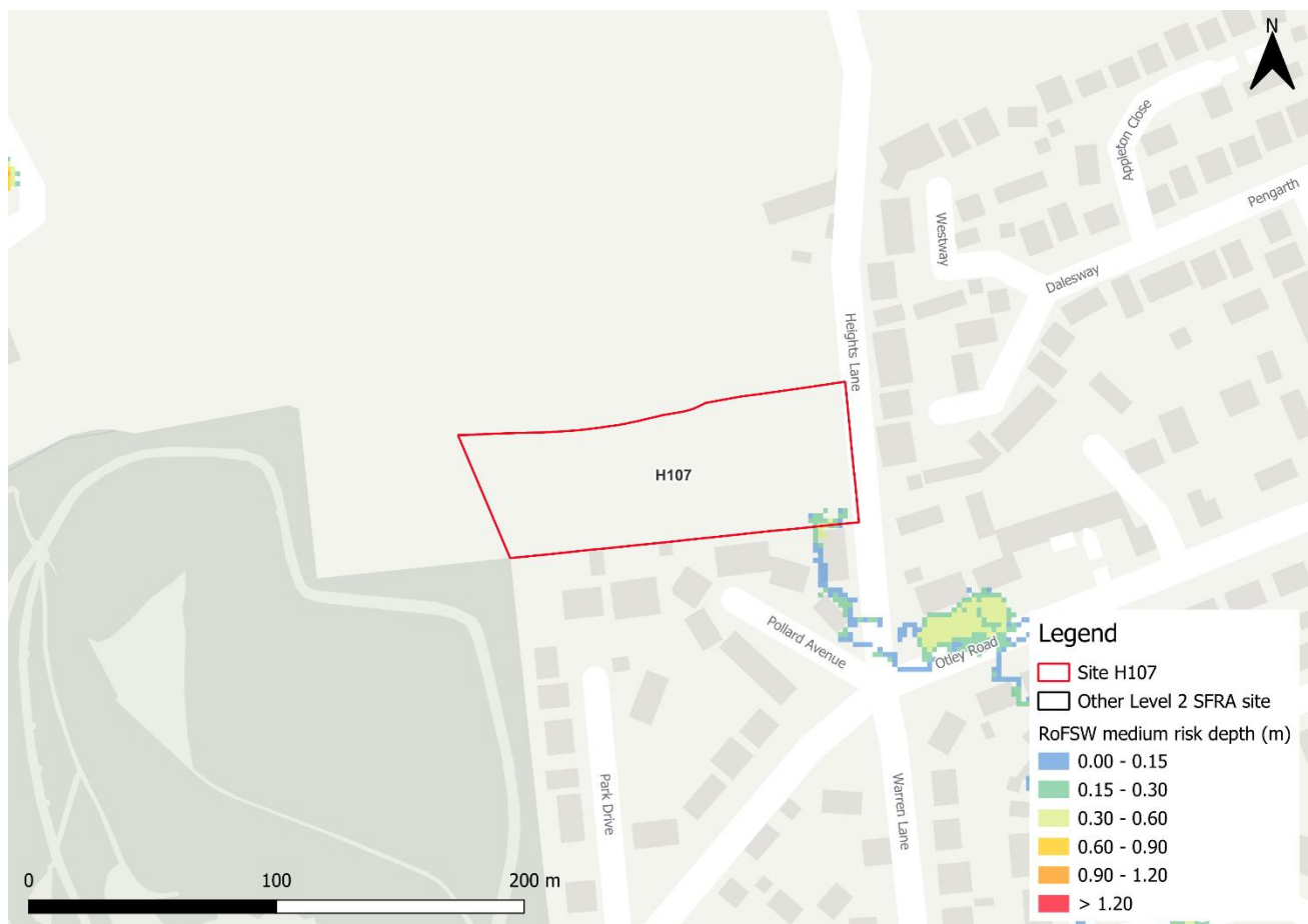
Figure 2-10: Medium risk event surface water flood depths within H107 (Risk of Flooding from Surface Water)
